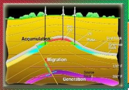
Seal (cap rock) is an impermeable rock that acts as a barrier to further migration of hydrocarbon liquids. Rooks that forms a barrier or cap above and around reservoir rock forming a trap such that fluids cannot migrate beyond the reservoir. The permeability of a seal capable of retaining fluids through geologic time is 10-6 to 10-8 darcies. A seal is a critical component of a complete petroleum system.
